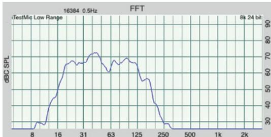
Fig.2 JL Audio Fathom f212v2s, uncorrelated pink noise before DARO, FFT display, 8Hz–2kHz, no low-pass filter, Salon2s off, full-range in-room response (80dB vertical range). Note 45Hz peak and 60Hz dip.
